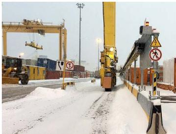
Montreal Gateway Terminals Partnership (MGTP) is the first Canadian container terminal facility to recently convert two rubber tire gantry cranes from diesel to electric power. In 2020, MGTP also purchased a total of 10 gantry cranes on electric wheels that consume 92% less fuel than diesel-fueled cranes.
